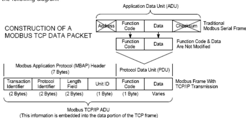
The MODBUS commands and user data are themselves encapsulated into the data container of a TCP/IP telegram without being modified in any way. However, the MODBUS error checking field (checksum) is not used, as the standard Ethernet TCP/IP link layer checksum methods are instead used to guaranty data integrity. Further, the MODBUS frame address field is supplanted by the unit identifier in MODBUS TCP/IP, and becomes part of the MODBUS Application Protocol (MBAP) header (more on this later).
